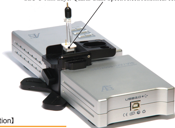
SEC-C Thin Layer Quartz Glass Spectroelectrochemical cell Kit
